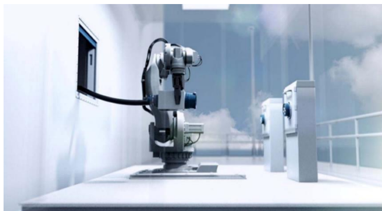
Figure 62: ABB IRB7600, an autonomous robotic arm used for charging 122
