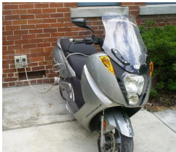
Figure 36: Home charging using a common wall socket 76
