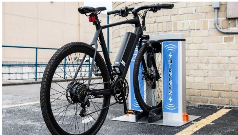
Figure 46: Electric bike wireless charging in a secure stand 95
