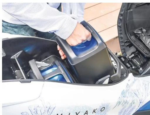
Figure 44: Remove a battery and replace it with a fully charged one 91
