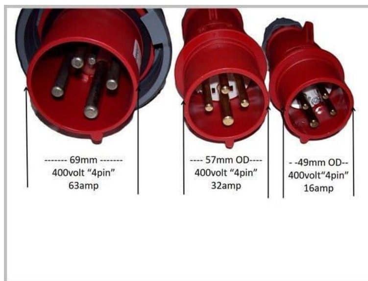
Figure 60: 3-phase AC plugs 121
