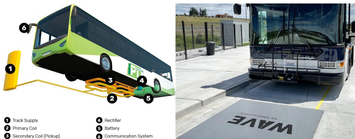
Figure 32: Model illustration of wireless charging on the left 62 and practical example of charging pad by Wave on the right 63
