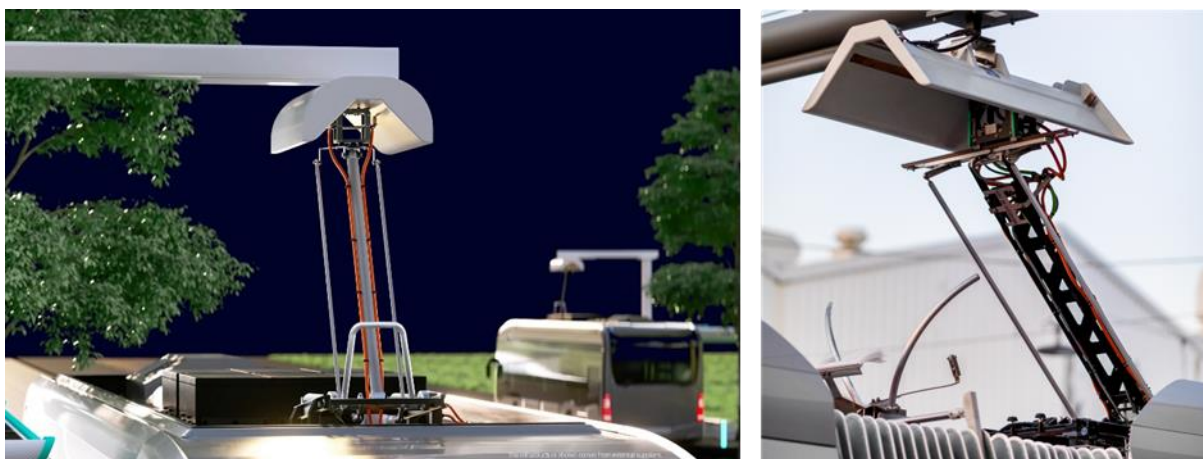
Figure 30: Example of roof-mounted pantograph: from SIEMENS 57 on the left and from SOLARIS 58 on the right
