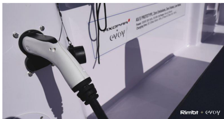
Figure 63: Shore charging Evoy leisure boat with Plug charger 123
