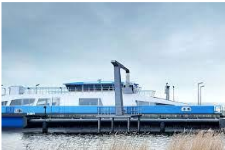
Figure 55: 'Zinus' charging solution for 'Singapore's first fully electric ferry route' 116
