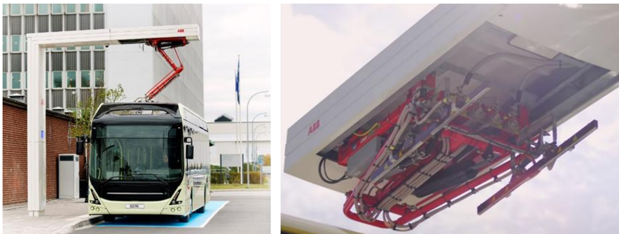
Figure 31: Inverted pantograph charging solution from ABB: e-bus during charging on the left 59 and retracted pantograph on the right 60
