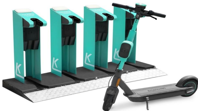
Figure 45: Kickgoing's electric scooter and its parking station with LG's wireless charging solutions 94
