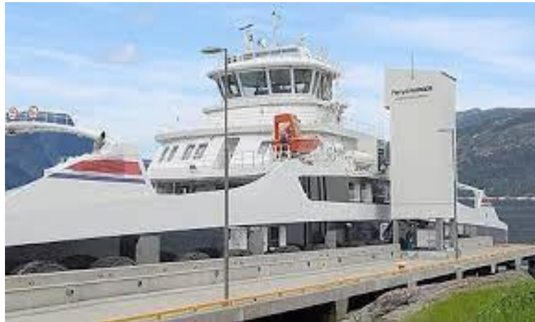
Figure 57: Stemann FerryCHARGER solutions for electric ferries, picture from Norway. 118
