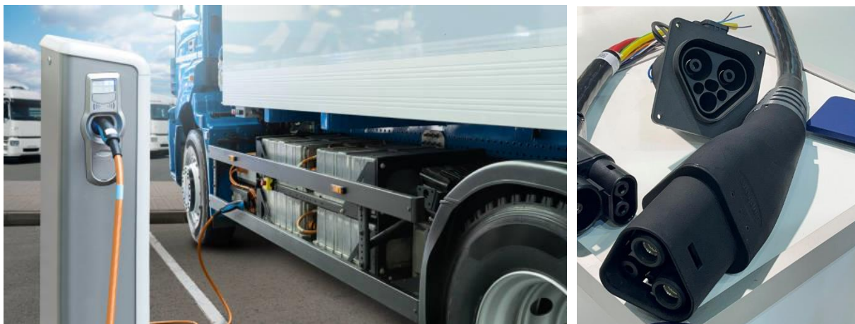
Figure 27: Wired charging of electric truck 51 on the left and port and cable for MCS 52
