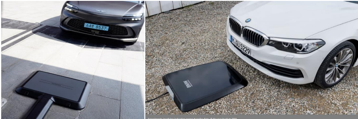
Figure 5: Wireless car charging on the left 9 and inductive charging on the right 10
