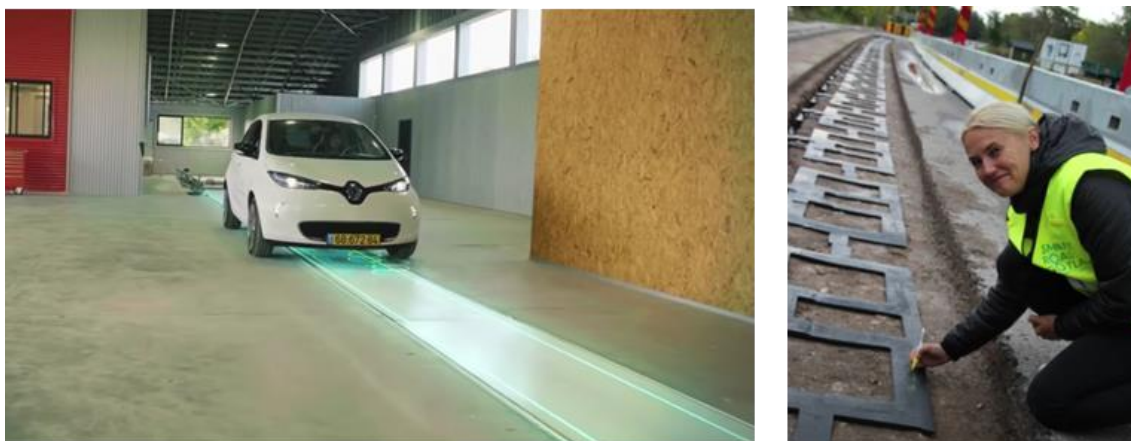
Figure 21: Wireless charging solutions by Israeli start-up Electreon on the right and piloting of wireless dynamic charging - coils underneath the road in Gotland on the left 36
