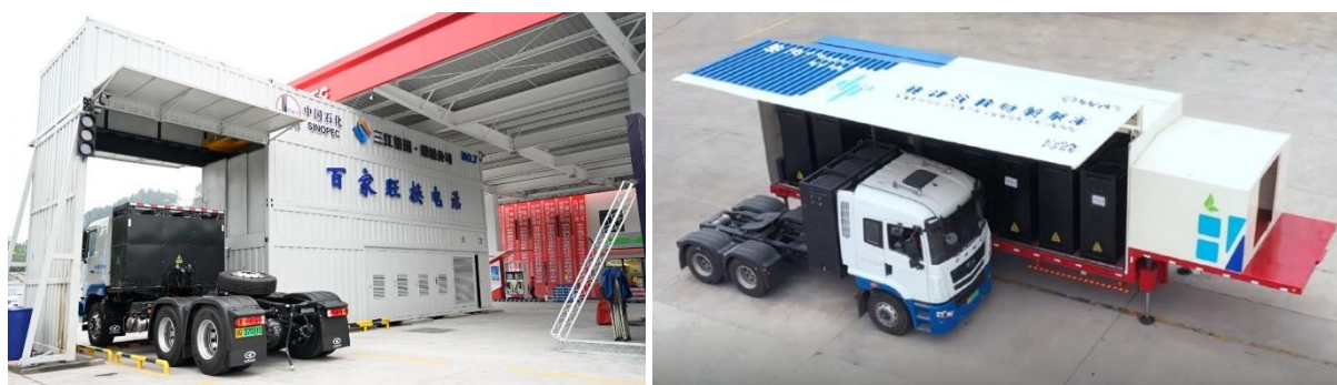
Figure 28: Sinopec's fixed battery swap station on the left 53 and SPIC's mobile battery swap vehicle (trailer) on the right 54
