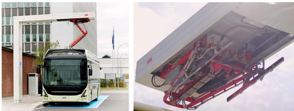
Figure 31: Inverted pantograph charging solution from ABB: e-bus during charging on the left 58 and retracted pantograph on the right 59
