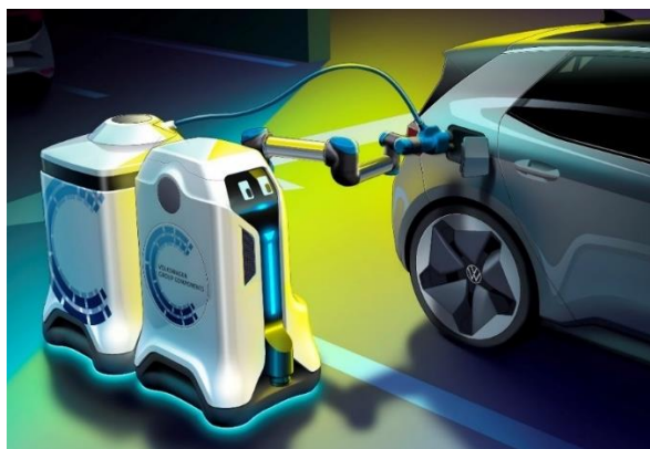
Figure 25: Automatic mobile charging robot by Volkswagen Group 43
