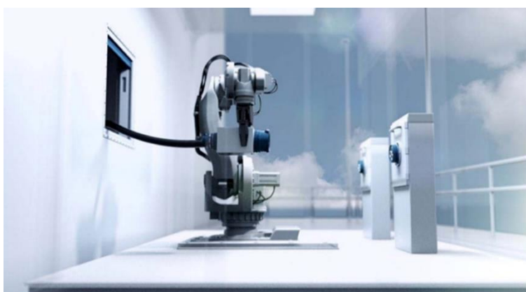
Figure 62: ABB IRB7600, an autonomous robotic arm used for charging 121
