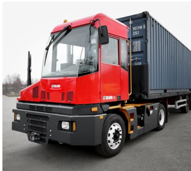
Figure 31. Terminal tractor with Lithium-ion batteries. Source: Kalmar
