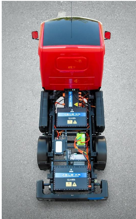
Figure 21: Placement of battery packs and electric motor of Tropos Motors utility vehicle 71
