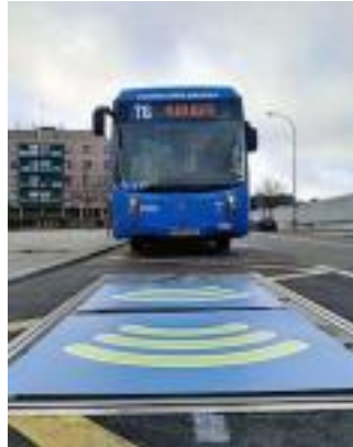
Figure 16: Wireless charging spot in Madrid located at the beginning and the end of the route
