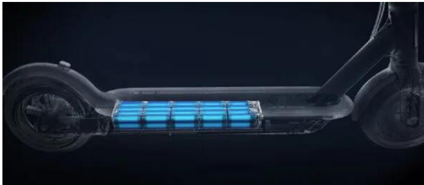
Figure 40: Example of storage of a battery pack in scooter 130
