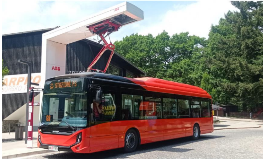
Figure 14: Iveco bus with pantograph charging 44
