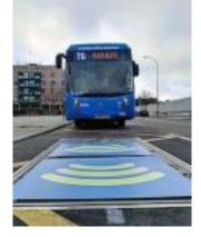
Figure 16: Wireless charging spot in Madrid located at the beginning and the end of the route
