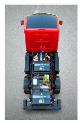
Figure 21: Placement of battery packs and electric motor of Tropos Motors utility vehicle<sup>71</sup>
