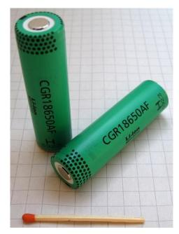
Figure 42: Example of battery cells used in a scooter battery pack<sup>131</sup>
