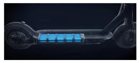
Figure 40:Example of storage of a battery pack in scooter<sup>130</sup>
