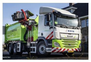
Figure 18: Example of an electric garbage truck<sup>53</sup>
