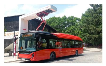
Figure 14: Iveco bus with pantograph charging<sup>44</sup>
