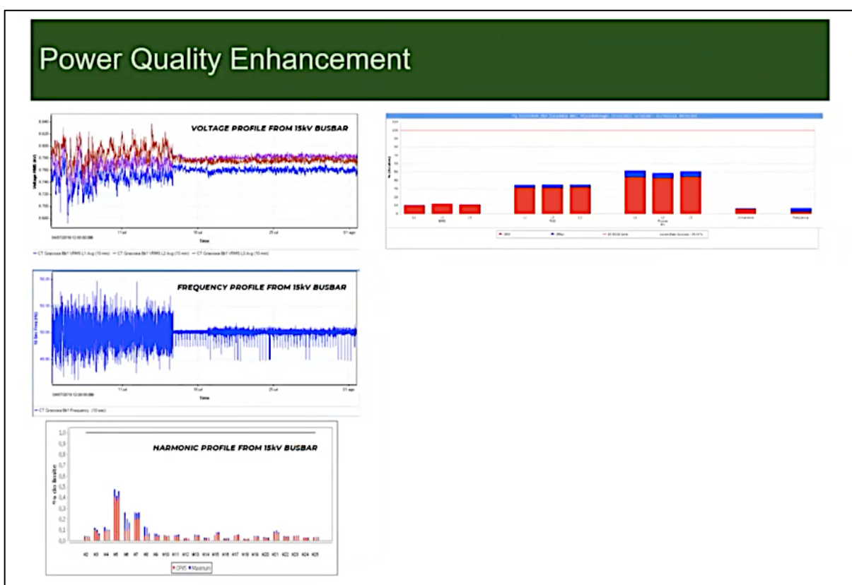
Figure 4. A screenshot of Mr Silva's slides. Various graphs show the effect of transforming from using only Diesel generators to renewables combined with BESS.
