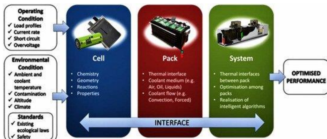
Figure 28. Battery Thermal Management System (BTMS)
